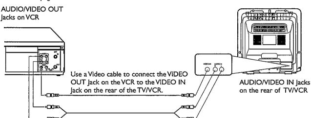
Use an Audio cable to connect the AUDIO OUT Jacks on the VCR to the AUDIO iN Jacks on the rear of the TV/VCR.
